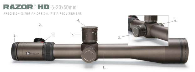
1. 3.9 IN. EYE RELIEF: The Razor<sup>™</sup> HD provides generous and consistent eye relief at all magnifications for faster target acquisition when shooting in a wide variety of positions and situations. The considerable eye relief eliminates eyestrain during extended viewing while protecting from recoil on large caliber rifles.
